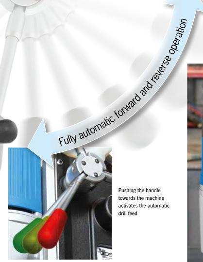
Pushing the handle towards the machine activates the automatic drill feed
